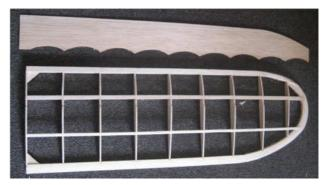
The tailplane is built in much the same way but I added an extra spar to make it stiffer and, of course, a moveable elevator by using a deeper
