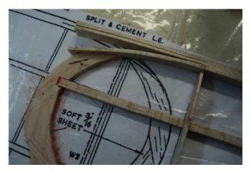
I started with the wings as they are the simplest and include a nice idea for bending the  $\frac{1}{2} \times 3/8''$  balsa LE to meet up with the tip formers – you split 'em so they form 3 thin easy to bend sections as you can see here and then glue them together again!
